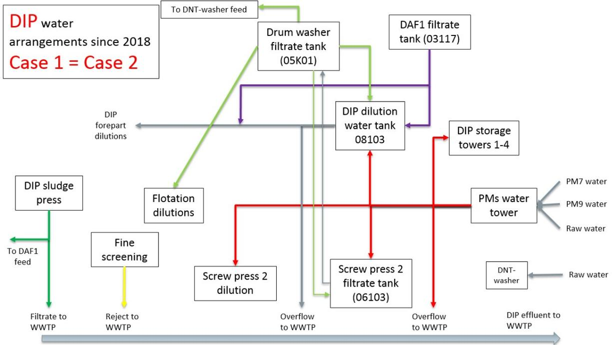
Figure 7. DIP white water system improvements (step 6 in water reduction action plan). Water circuit arrangements in deinking plant in Case 1 and Case 2.
