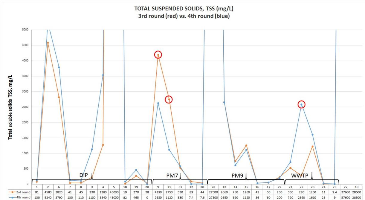
Figure 3. Total suspended solids (TSS) levels before (red line) and after (blue line) the first actions to reduce water consumption in Essity Nokia tissue mill were conducted.
