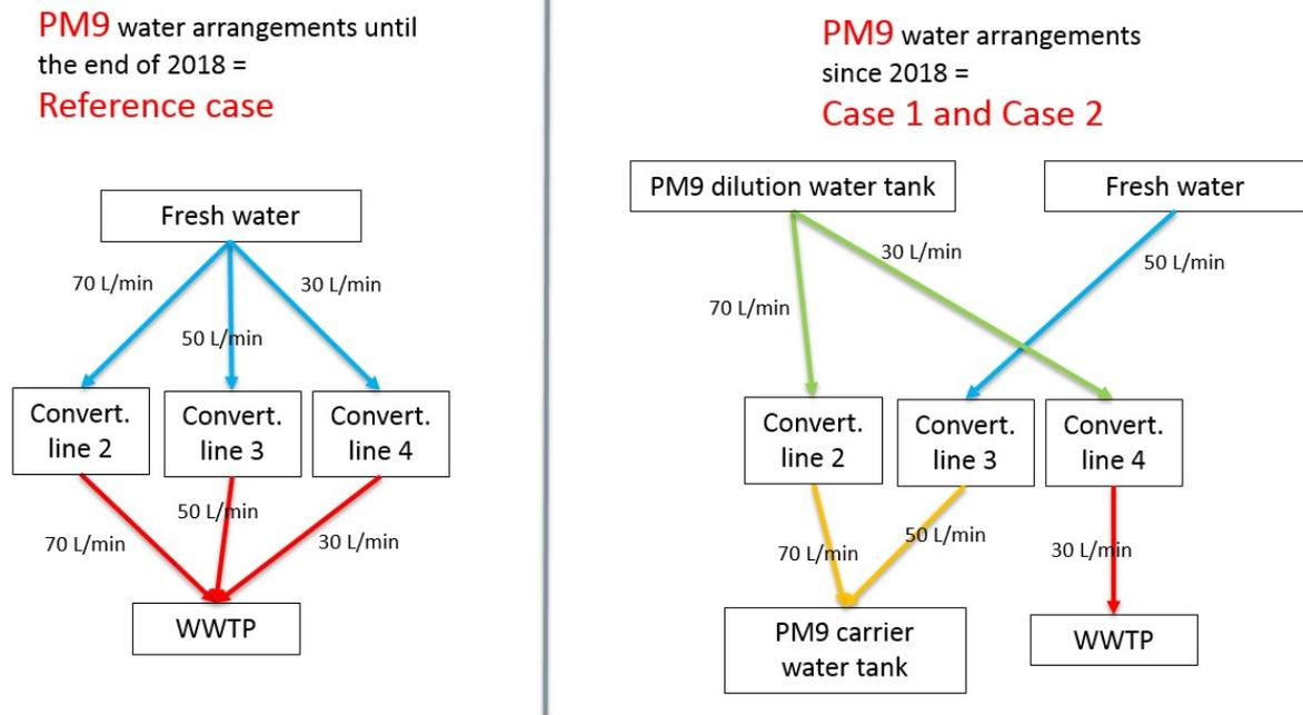
Figure 9. Actions to reduce water consumption in PM9 (steps 4 and 5 in the water reduction action plan): i) dustwashers in converting lines 2 and 4 changed from fresh water to PM9 white water and ii) reuse of dustwasher waters from converting lines 2 and 3 instead of directing to WWTP.
