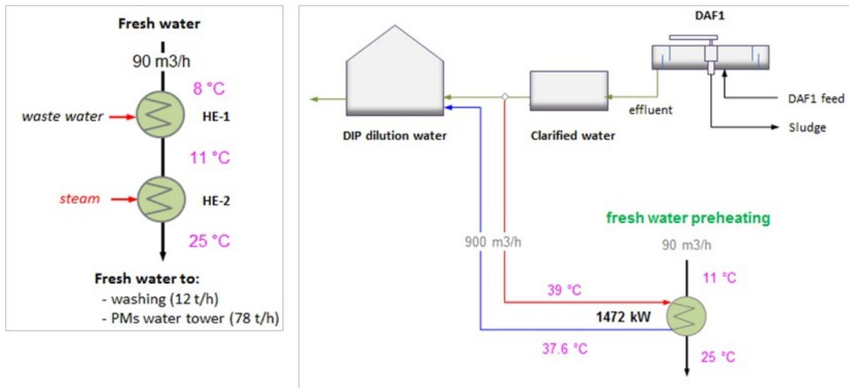
Figure 19. Existing situation DIP (left) and proposed modification (right) for **option-1**.
