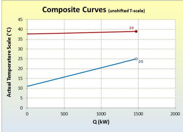
Figure 18. Using clarified DAF-1 waters for preheat fresh water DIP (option 1).
