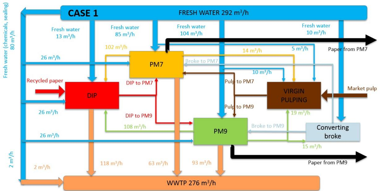
Figure 11. Case 1: Water balance in Essity Nokia mill since 2018 when first actions to reduce the fresh water consumption have been executed.
