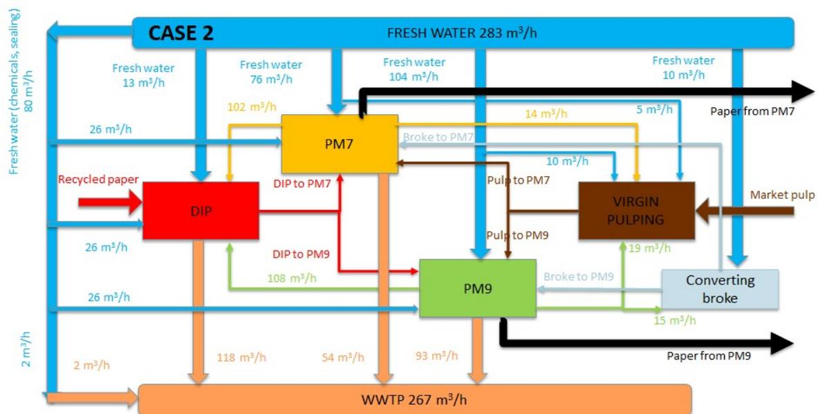
Figure 12. Case 2: Water balance in Essity Nokia mill since 2018 when first actions to reduce the fresh water consumption have been executed and Valmet's CR-filter implemented to PM7 to produce clear permeate from disc filtrate.
