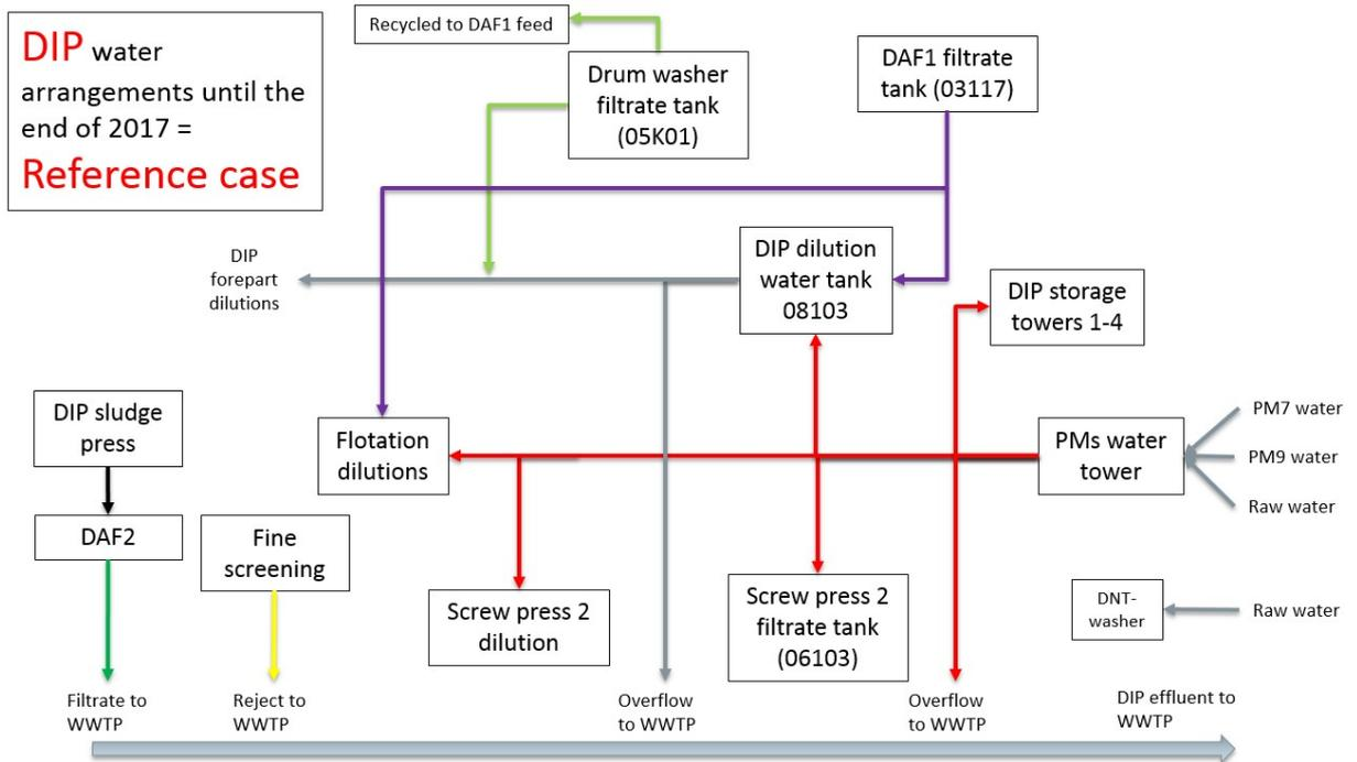
Figure 6. Water circuit arrangements in deinking plant until the end of 2017 before any DIP water system improvements have been executed (Reference case).
