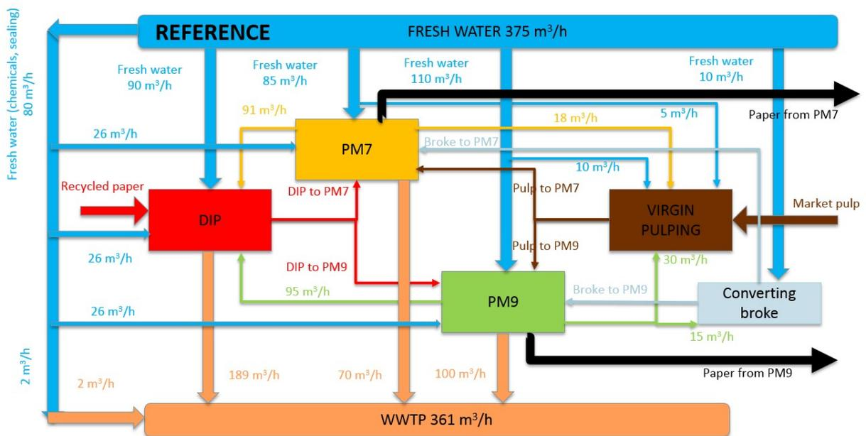
Figure 10. Reference case: Water balance in Essity Nokia mill until the end of 2017 when no actions to reduce the fresh water consumption have been executed.
