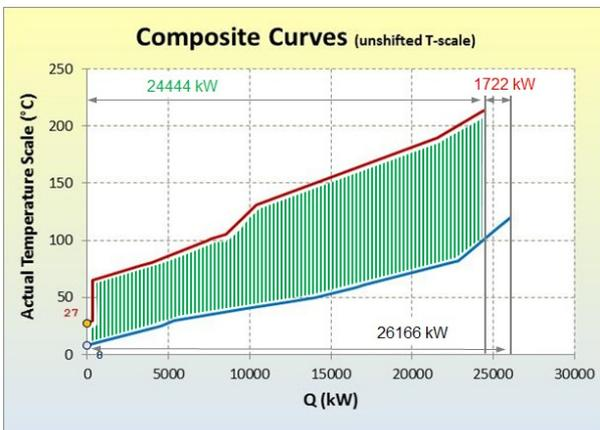
Figure 16. Composite curves for the Reference case of the Nokia mill.
