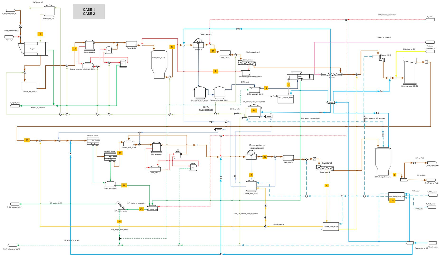
Figure 25. Essity Nokia tissue mill – Deinking plant for Case 1 and Case 2.
