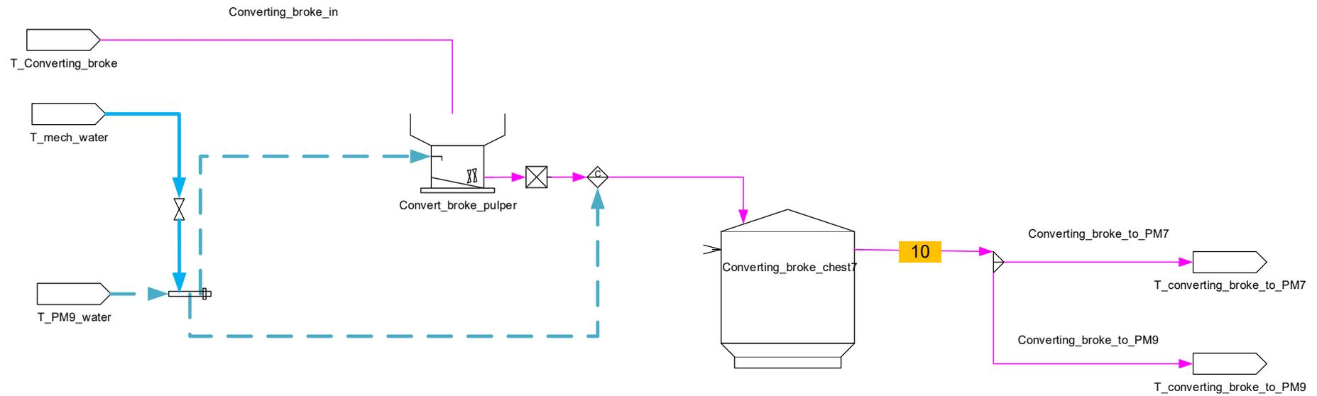
Figure 34. Essity Nokia tissue mill – Converting broke pulping for Reference case, Case 1 and Case 2.
