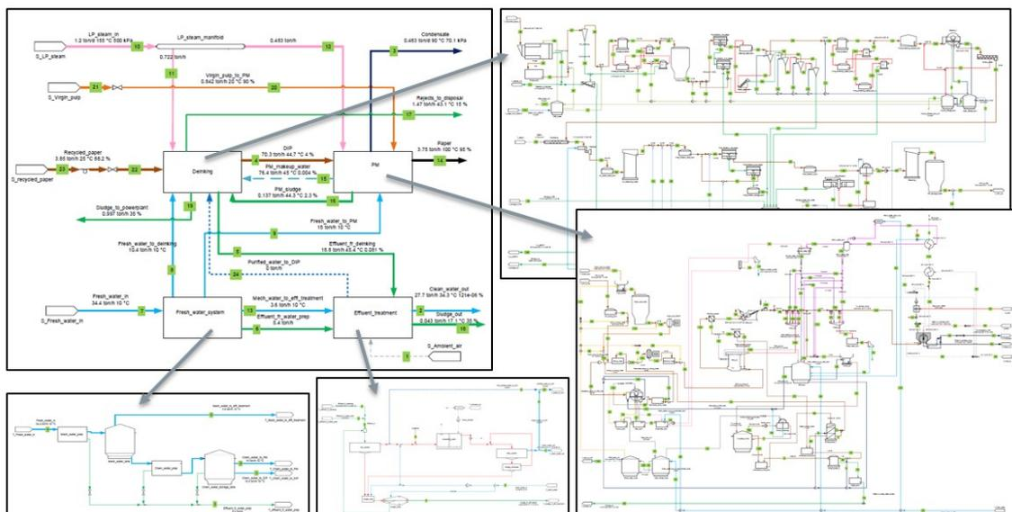
Figure 5. Flowsheet of the generic BAT-based tissue mill model.
