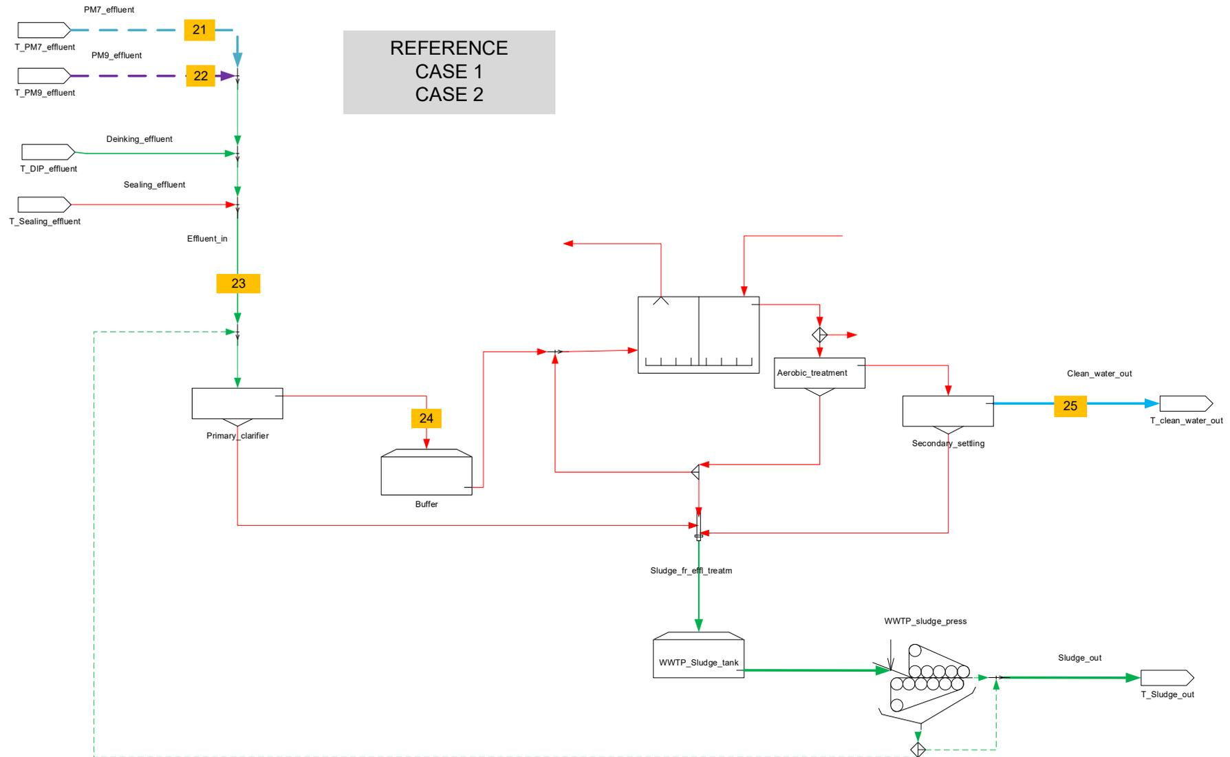
Figure 31. Essity Nokia tissue mill – Waste water treatment plant for Reference case, Case 1 and Case 2.
