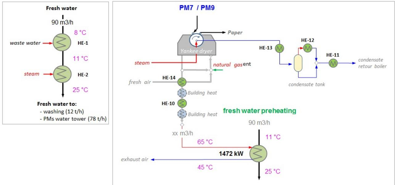
Figure 21. Existing situation DIP (left) and proposed modification (right) for **option-2**.
