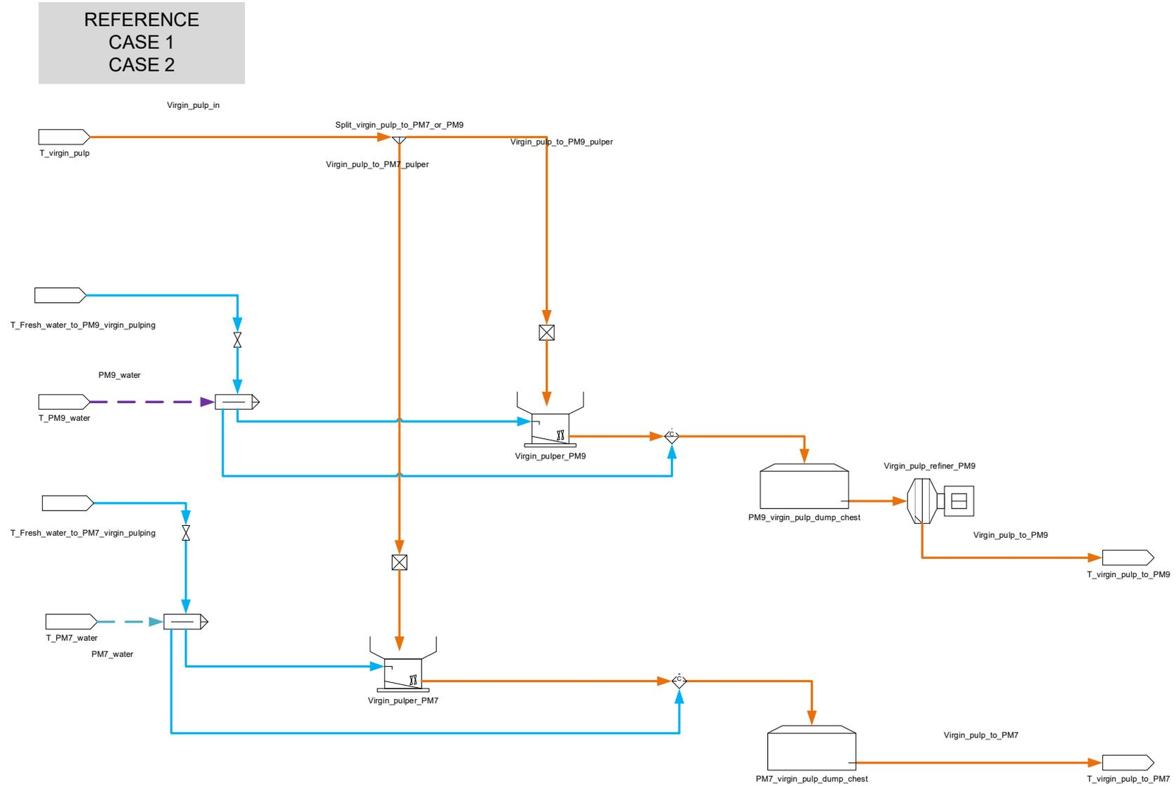
Figure 33. Essity Nokia tissue mill – Market pulp pulping for Reference case, Case 1 and Case 2.
