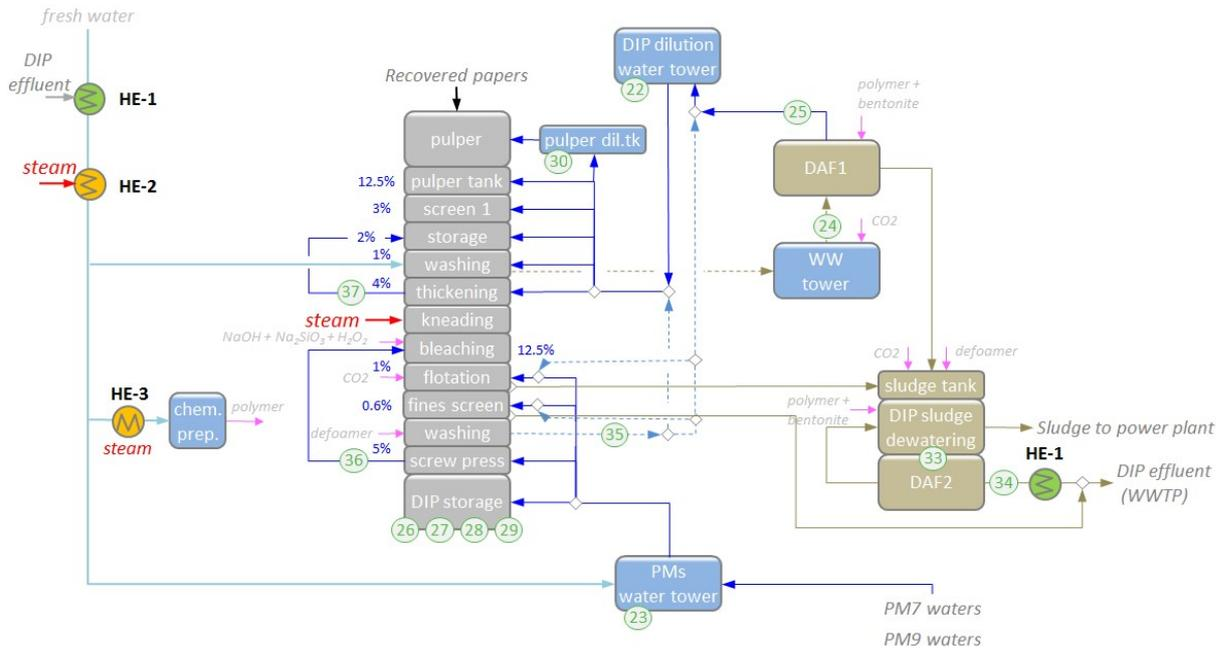
Figure 13. Simplified block diagram of DIP section in Reference case with locations of existing HE's.
