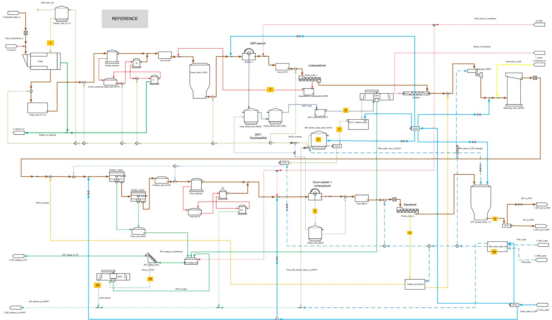
Figure 24. Essity Nokia tissue mill – Deinking plant for Reference case.
