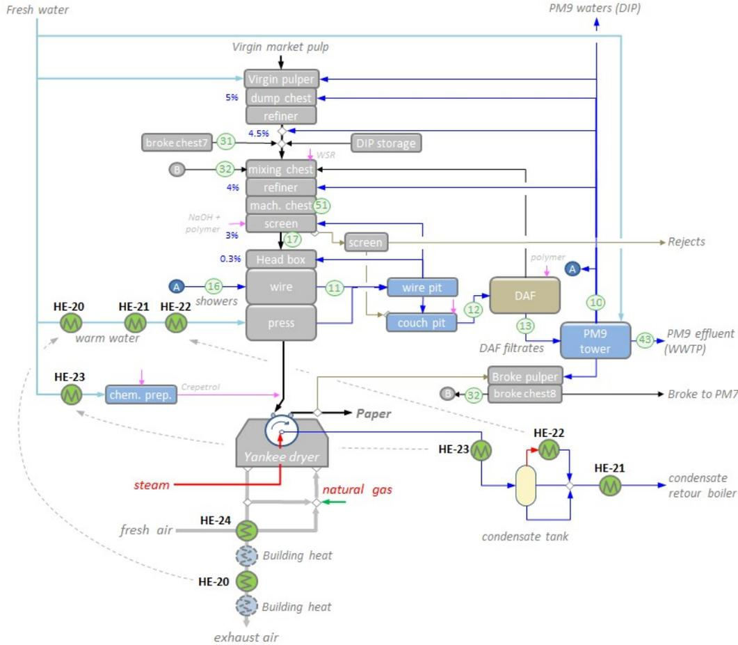
Figure 15. Simplified block diagram of PM9 in Reference case with locations of existing HE's.
