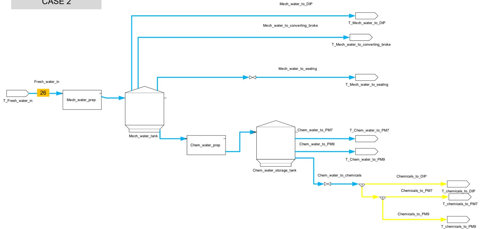
Figure 32. Essity Nokia tissue mill – Fresh water production for Reference case, Case 1 and Case 2.
