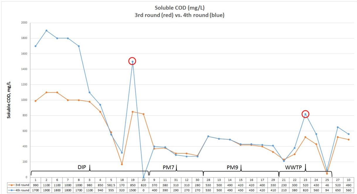
Figure 4. Soluble COD levels before (red line) and after (blue line) the first actions to reduce water consumption in Essity Nokia tissue mill were conducted.
