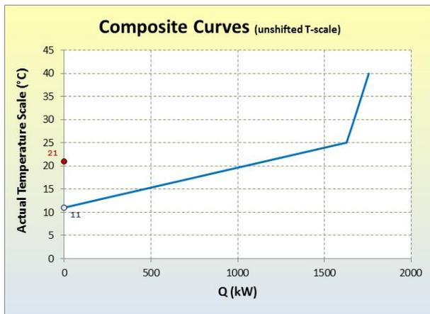
Figure 17. Composite curves without existing heat integration.
