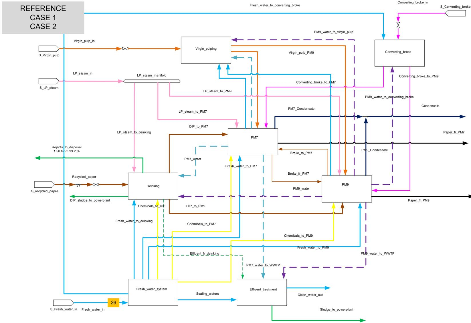
Figure 23. Essity Nokia tissue mill - Main flowsheet for Reference case, Case 1 and Case 2.
