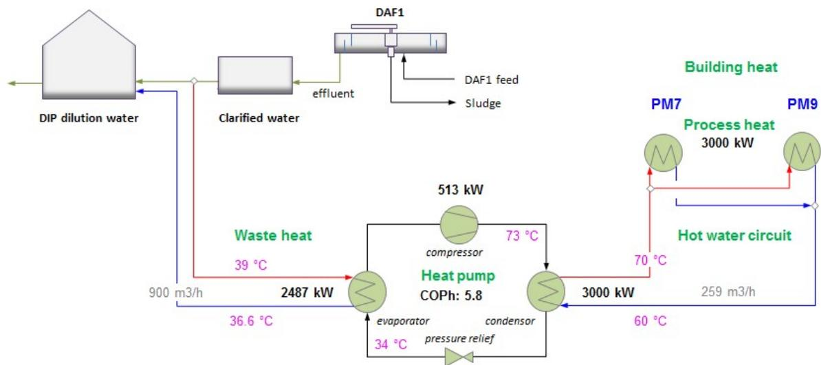
Figure 22. Hot water generation with a heat pump by using 'waste heat' from the DIP.
