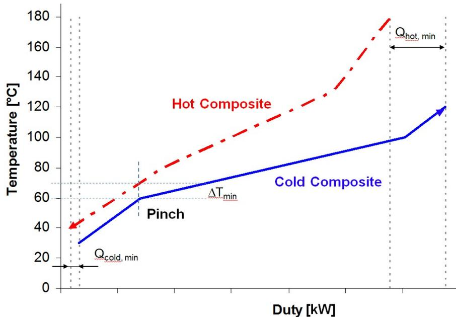
Figure 2. The basic principle of pinch analysis.
