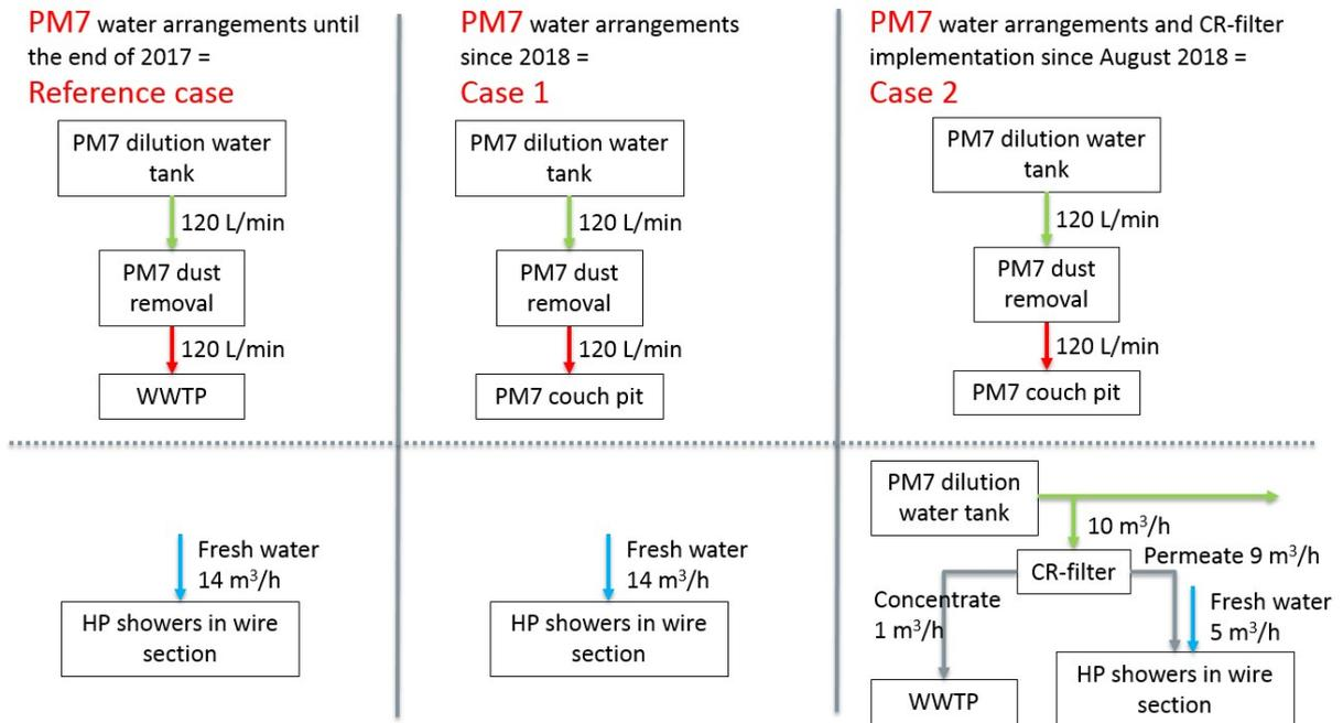
Figure 8. Actions to reduce water consumption in PM7 (steps 4 and 5 in the water reduction action plan): i) reuse of PM7 dust removal waters instead of directing to WWTP and ii) implementation of Valmet's CR-filter to produce clear permeate from white water to be used as HP-shower water in wire section.
