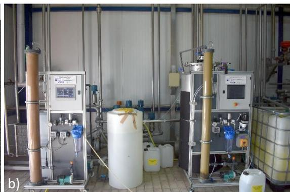
The aaMBR pilot plant: a) A 3-D view of pilot design. b) Front view of operating pilot; the anaerobic MBR unit at the right-hand side.
